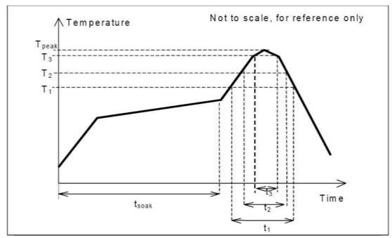
This profile is the minimum requirement for evaluating soldering heat resistance of components. Heat transfer method used for reflow soldering is hot air convection. The actual air temperatures used to achieve the specified profile is higher and largely dependent on the reflow equipment.
